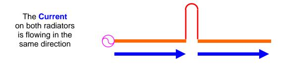
You can even stack them with four half wave radiators to get 6 dB gain over a single half wave length Zepp J-Pole antenna. Now that's something from an omni antenna.
