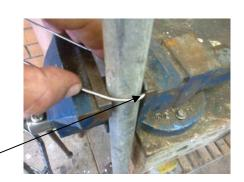
The above image of a 2.4 mm 316 grade stainless steel welding rod I purchased for the job at hand with the mid-point marked with a felt tipped pen and bent in the middle point around a piece of pipe as seen in the image above.
